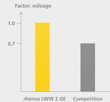
*rhenus LWW 2 GE performed impressively in a practical test, with a significantly lower friction coefficient. In terms of the mileage, the wheelset bearings covered around 30% more mileage with rhenus LWW 2 GE than with a comparable grease from a competitor.\**
